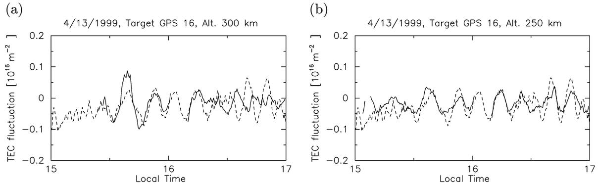
**Figure 3:** A feasibility test to estimate the TEC fluctuation along the ray path of a target satellite by using the TEC data observed by another GPS satellite. Dashed curve is the "true TEC" observed by the target GPS satellite No.16, while solid curve is the "estimated TEC" which are the averages of the TEC values by the satellite No.14 at surrounding points. The TEC fluctuation is assumed to be localized on the (a) 300 km and (b) 250 km surface.
